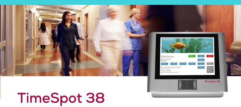
The TimeSpot 38 is a modern touchscreen punch clock designed for 24/7 operation, year after year. It runs on the Linux operating system, ensuring exceptional reliability, and features an integrated web browser to display your system's time-tracking web application. The device supports multiple identification methods, including fingerprint recognition, RFID fob, pin-code, YubiKeys and Smart cards.
